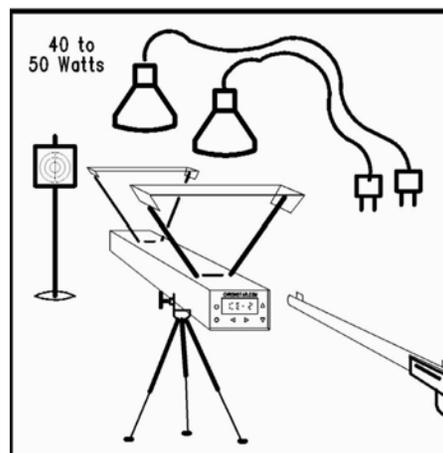
Install diffusers as shown and two 40 to 60 Watts light bulbs about 2 to 4 feet high from the diffusers. If you use flood lights, then a single 100-Watt bulb, 4-feet above the center of unit would be sufficient.
