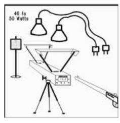
Install diffusers as shown and two 40 to 60 Watts light bulbs about 2 to 4 feet high from the diffusers. If you use flood lights, then a single100-Watt bulb, 4-feet above the center of unit would be sufficient.
